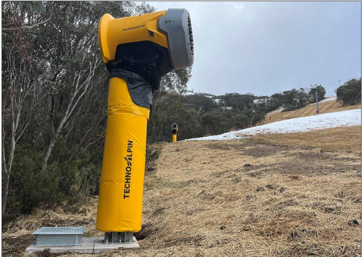
Figure 5 | Example of T110 type snowmaking fan gun and pit (Source: Applicant's Documentation)
