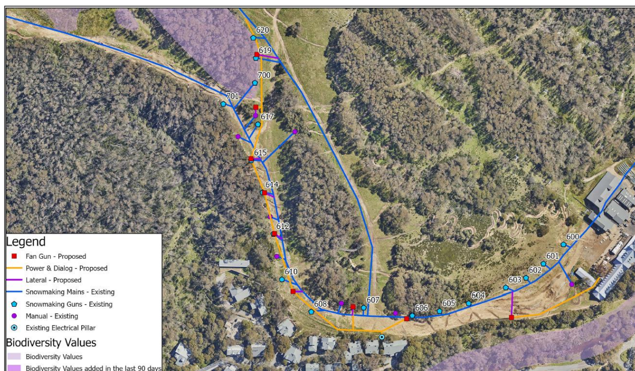
Figure 4 | Lower Supertrail area showing existing and proposed snowmaking and services infrastructure (Source: Applicant's Documentation)
